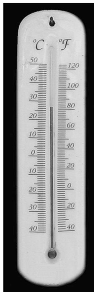
Fig. A1.1 Thermometer with two temperature scales (Photo W.H.B.)
