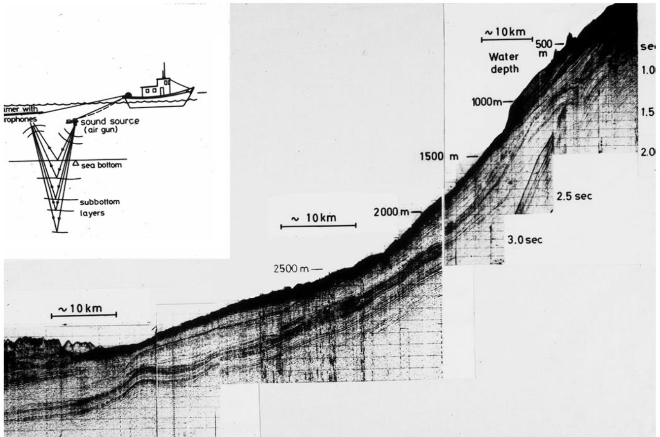
**Fig. 3.14** Submarine mass movements off Dakar (Senegal, NW Africa). Air gun record of Meteor Cruise 25/1971. Thickness of slide is ca. 200 m. (Note vertical exaggeration.) *Insert:* air gun system with air
