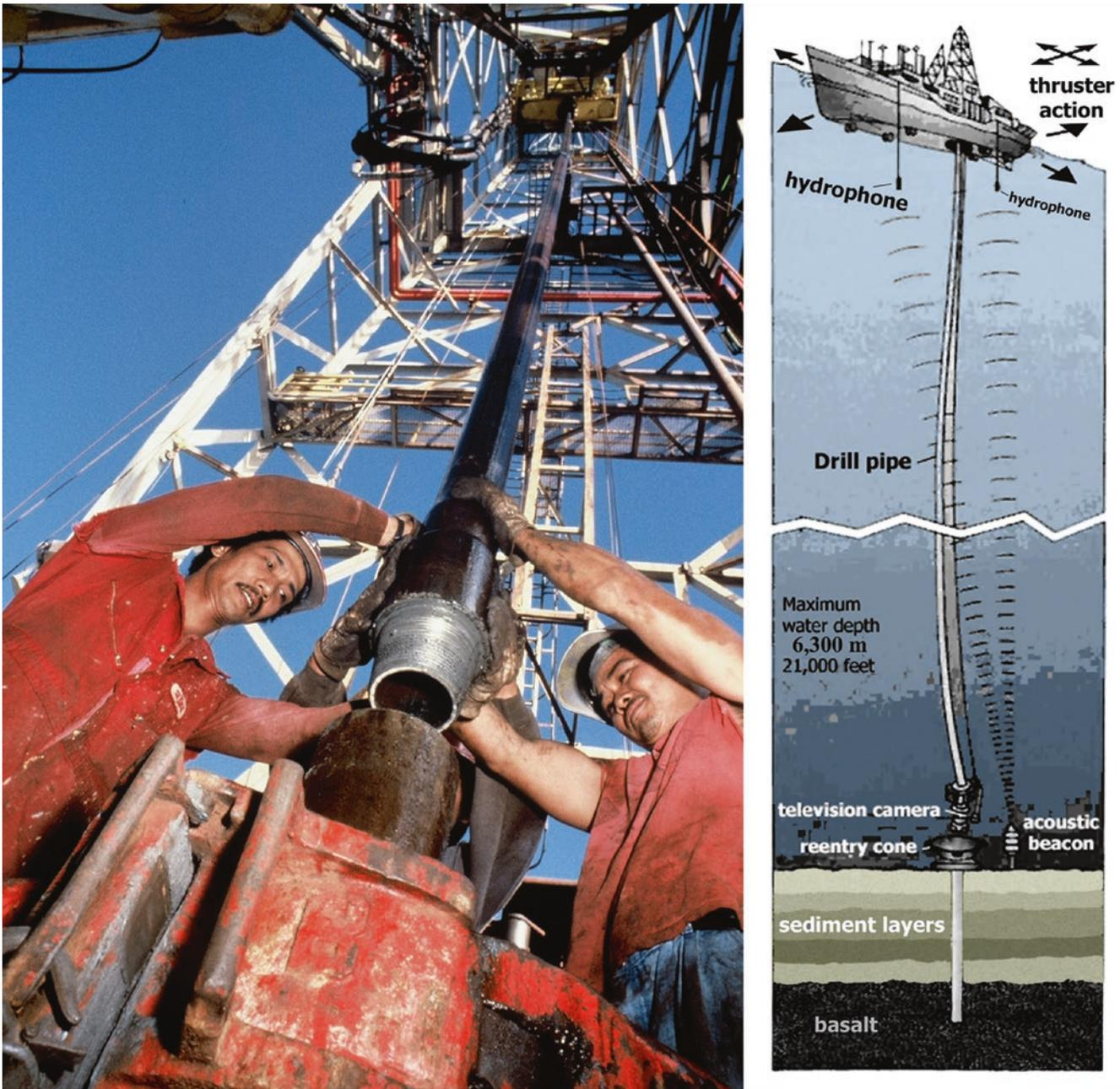
**Fig. 12.5** Retrieving information on Cenozoic history from the seafloor. The chief source of information is drilling from a vessel (here: the JOIDES Resolution is a vessel originally used by BP in commercial
